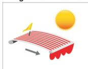
If the light intensity exceeds the set grade for 10 minutes continuously, a Down order is given to the motor and the awning opens automatically.
