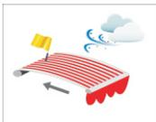
If the wind speed exceeds the set grade for 6 seconds continuously, an Up order is given to the motor and the awning will close automatically.
