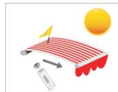
If the wind speed falls below the set grade for 30 seconds continuously, the sensor sends signals to the motor and activates the control by emitter and light sensor.
