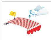
As long as real wind speed is higher than the set grade, you can't open the awning by any means (manual control, emitter control and light sensor are invalid).
