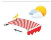
If the light intensity below the set grade for 10 minutes continuously, an Up order is given to the awning and the awning closes automatically.
