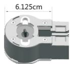
The length of aluminum track = the length of entire rail - the length of transfer box\*2
